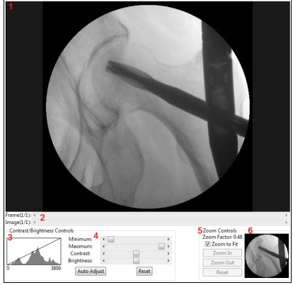
When a series is selected in the Browser, its first image is displayed in the Viewer. The Viewer has a viewing area on top (1), and a control panel at the bottom. Users can use the appropriate scrollers ((2)) to iterate over frames of an open image or images of a series. The left part of the control panel shows a graph of image data statistics (3) and controls to adjust maximum/minimum/contrast/brightness of the image (4). On the right, a mini map of the image (6) and controls for zooming (5).
